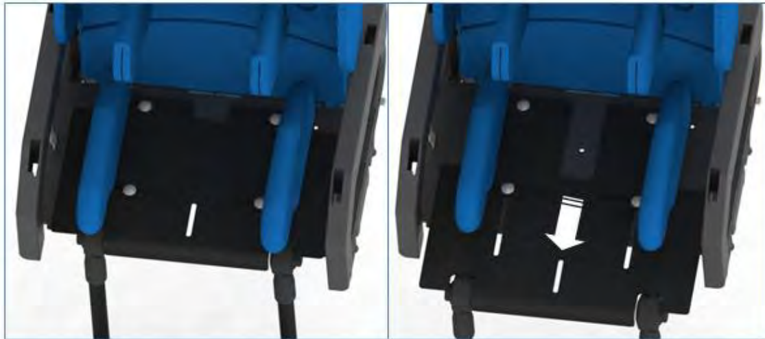
Fig. 20 Seat depth adjustment
