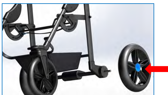
Fig. 12 Removal and installation of rear wheels
