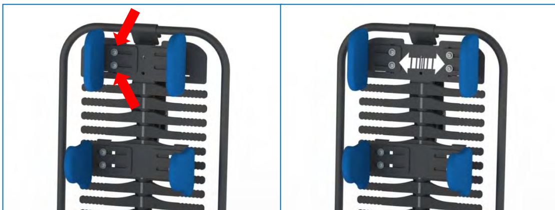
Fig. 26 Head supports adjustment
