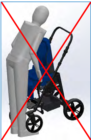
Fig. 5 Incorrect manner of moving the buggy
