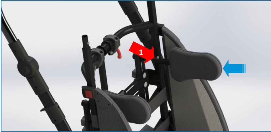
Fig. 10 Chest supports installation
