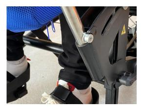
B. Push the knee block towards the user. When it's in the right place lock it with a handle/screw on the side.
